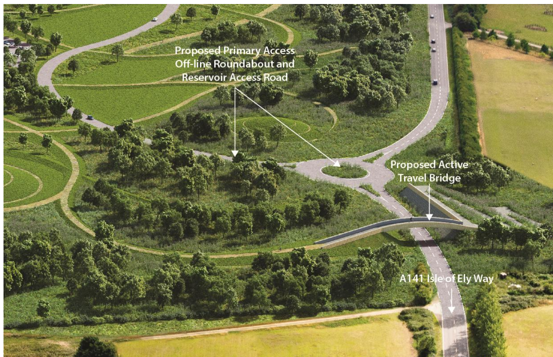
Figure 7.22: Three-armed roundabout access and proposed active travel bridge (view southbound from Wimblington)
