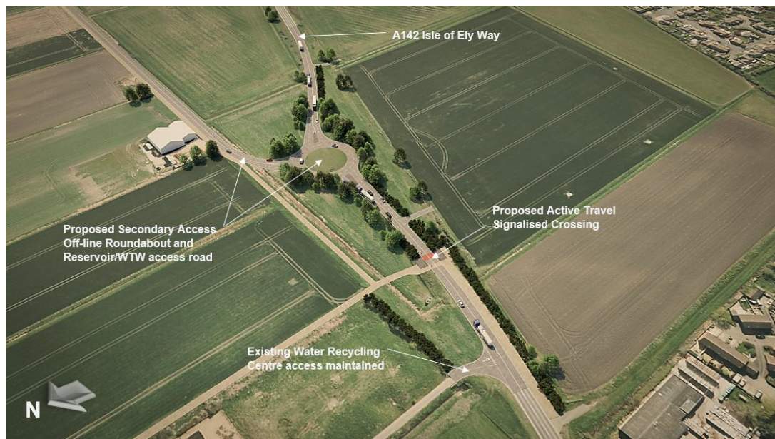
Figure 7.23: Three-armed roundabout access to the reservoir and water treatment works (view eastbound from Chatteris)
