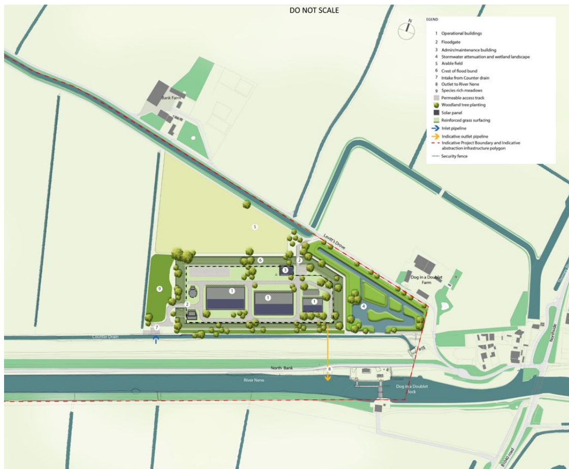
Figure 6.7: Our proposals near Whittlesey. Area for raw water infrastructure to abstract water from the Counter Drain (Nene) and discharge it into the River Nene.
