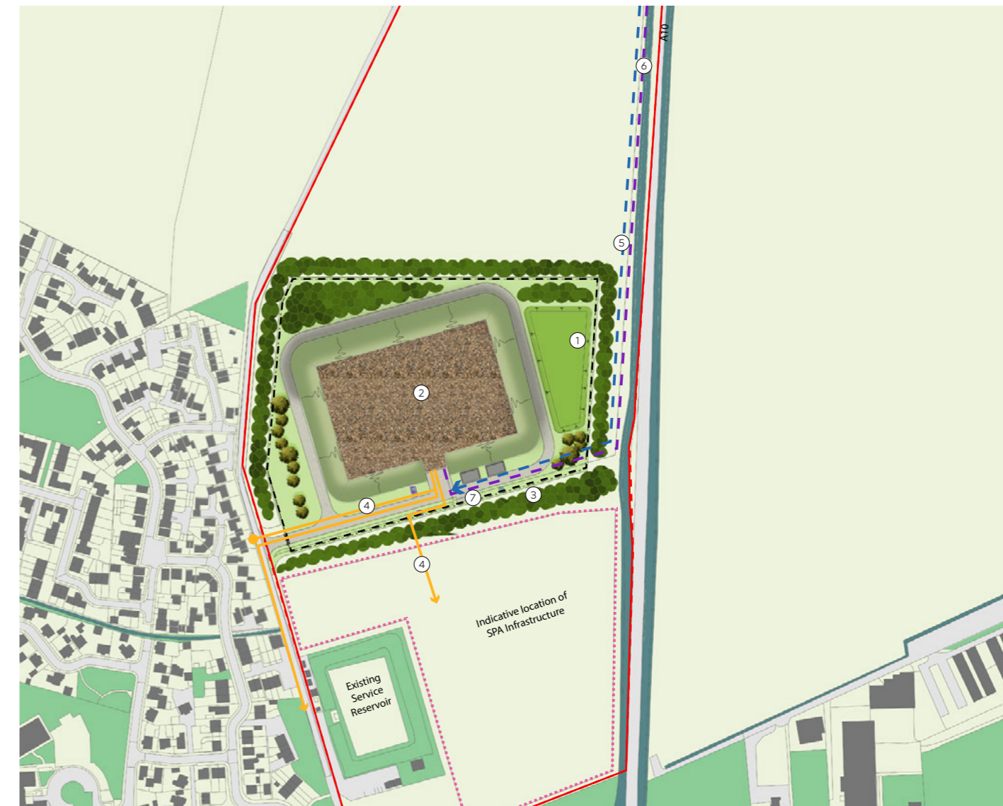
Indicative plan, within the identified area, for storing treated water for supply to Anglian Water customers, at Bexwell.
